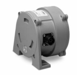
The IT9232 delivers incline position feedback via RS232 or RS485 serial communication to your data acquisition or controller system. The heart of this inclinometer is a magnetically-damped pendulum coupled to a conductive plastic precision potentiometer.
