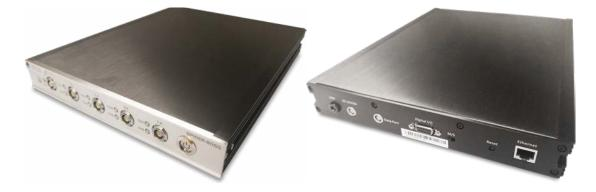
The Spider-80SG is a high precision, general purpose data acquisition device featuring strain gage capability.
